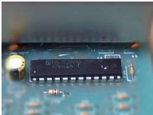
Figure 6. You can use a 20V8 or 16V8 PLD device for U1. Make sure you put a jumper wire to short J1 holes if a 16V8 is used.
