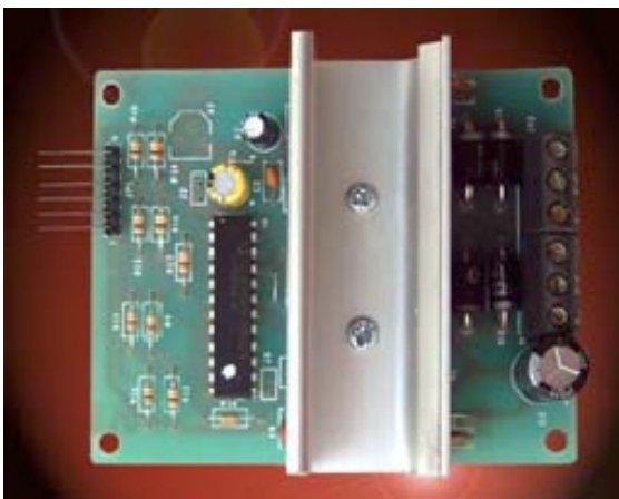
Figure 1. e-Gizmo's Universal PWM driver circuit looks surprisingly simple. All the PWM circuit complexities are hidden inside the driver IC itself, making it possible to come up with a high performance driver that is easy to build, easy to use, and very affordable!
