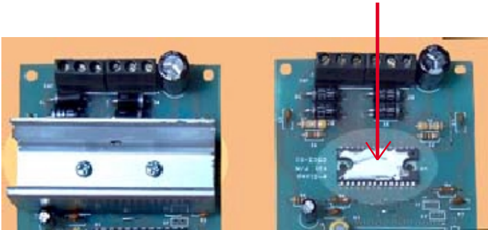
Figure 4. Apply a thin layer of heat sink (thermal) compound on top of U2 (right) before you mount the heat sink.
