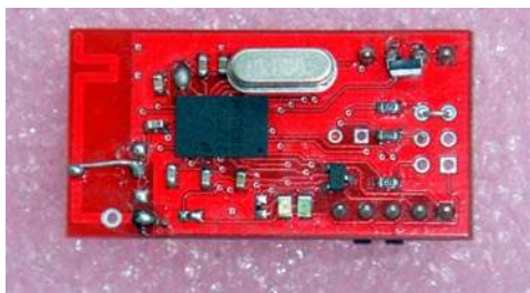
Figure 1. The EGBT 9830 BlueTooth module is based on National Semiconductor's high performance BlueTooth chip LMX9830.
