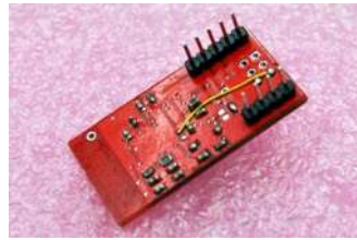
Figure 2. EGBT 9830 terminals are single row headers with pitch and spacing that will allow you to mount it on a breadboard, prototyping board, or even on an IC socket.
