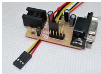
Figure 6. Use as short as possible wires for the debug connector. In this setup, red = +3v3, black = gnd, yellow = debug.
